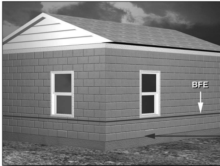
Figure 7 Technique 1 – Extend the walls of the house upward and raise the lowest floor.
